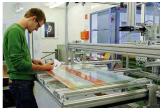
Fig. 2: The filling process for a dye solar module with dimensions of 60 cm x 100 cm. Together with Fraunhofer IAO, we have developed and constructed an industrially relevant production unit for this process.
