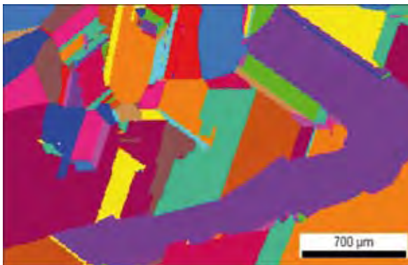
Fig. 1: Measurement of crystal orientation by electron back-scatter diffraction (EBSD) in the scanning electron microscope. We can determine the crystal orientations in multicrystalline silicon with high spatial resolution, based on automatic evaluation of interferences between the electrons that are diffracted by the crystal lattice.
