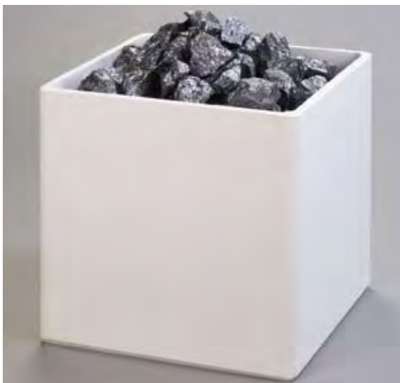
Fig. 1: Crystallisation from silicon feedstock covering a wide quality range is our first research focus within the silicon value chain. The photo shows feedstock in a quartz crucible for a block weighing 85 kg. The crystallised block is illustrated in the introduction to the chapter on silicon photovoltaics. (see page 42).
