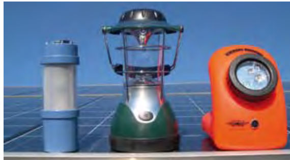
Fig. 1: Different types of photovoltaically powered LED lamps. The models on the left and the right are each equipped with a single high-power white LED; the centre model contains many low-power LED's. During the day, the integrated NiMH rechargeable battery is charged by a small photovoltaic module with app. 5 W power. Depending on the dimensions, illumination times of 3 to 8 h during the night are achieved. The quality of the photovoltaic modules and the rechargeable batteries is relatively good, the average deviation from the rated value is minus 10 %.
