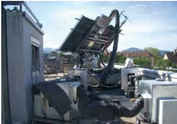
Fig. 1: Air collector test stand, installed for performance measurements on the roof of Fraunhofer ISE. The collector mounted on the solar tracker is visible, as are the individual components of the test circuit in the foreground: two fans (on the inlet and outlet sides), two volume flow meters and the heat exchanger, which defines the operating temperature of the air collector via a controlled thermostat during the efficiency measurement.
