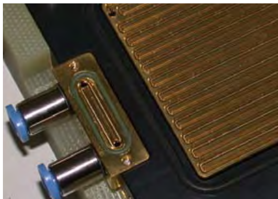
Fig. 1: Anode flow field of a fuel cell with the reference electrode configuration, which allows separate measurement of impedance spectra for the anode and the cathode.
