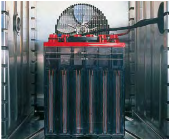
Fig. 1: In the climatic chamber, not only efficiency and capacity but also the aging and charging performance of storage batteries can be investigated under variable conditions.
