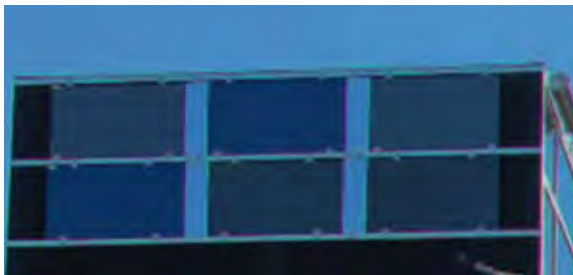
Fig. 1: Insulating glazing units from different product families have been mounted in front of a black wall of the rotatable container on the roof of Fraunhofer ISE. At an incidence angle of 20 °, the colour difference between the various windows is just perceptible.
