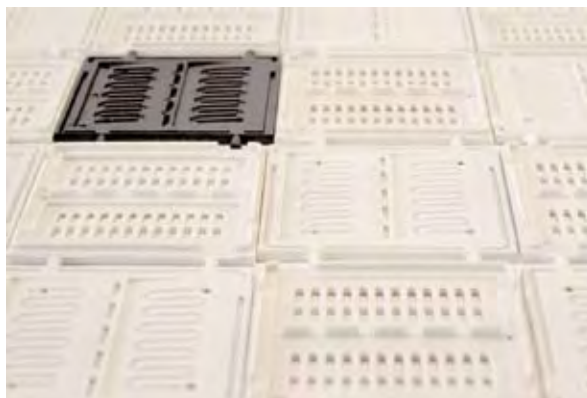
Fig. 2: Planar fuel cells as far as the eye can see: Large production volumes thanks to injection-moulding technology. Applications for the small power supplies can be found wherever small industrial and consumer devices need to be operated for weeks and months independently of the grid. The longer the required operating time, the more advantageous it is to use methanol as a fuel rather than conventional battery-based storage units.
