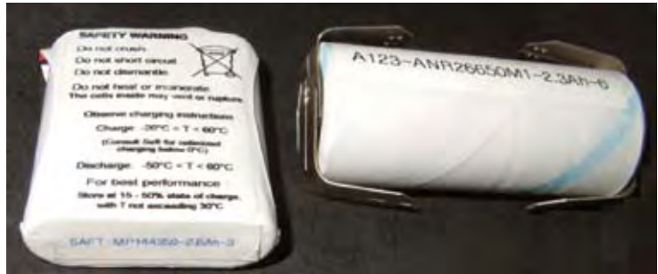
Fig. 1: The photo shows two of the lithium batteries that were modelled within the German-French co-operation project, EMSIS. The negative electrode consists of carbon for both batteries; the positive electrode is made of \text{LiCoO}_2 for the left-hand cell and of \text{LiFePO}_4 for the right-hand cell. The developed model can be used for batteries of different capacities and technological types.
