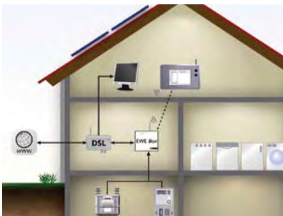
Fig. 2: Structure of the smart metering system. The EWE box serves as the central energy gateway and processes the meter data. In future, further value-added services such as distributed load management are planned for the box.
