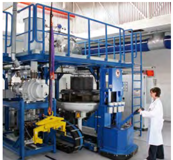
Fig. 2: We can study different approaches to directional solidification with individual process control in our crystallisation unit, where blocks with variable dimensions from 20 kg to 250 kg can be solidified. In the photo, the open furnace can be seen with a graphite support crucible for a Si block weighing 85 kg.
