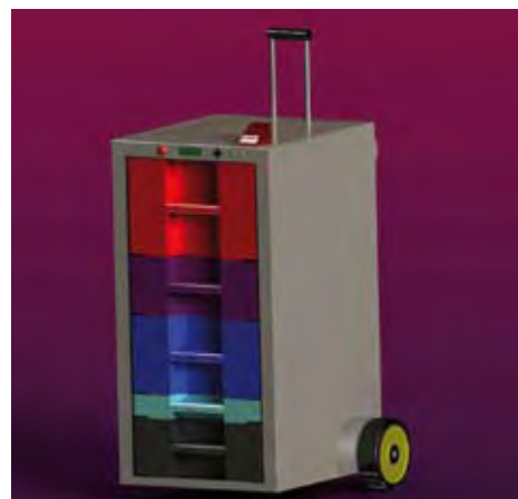
Fig. 4: 3D view of the modular RFCS. The reformer module is located at the top (red), with the FC module below it (violet). The other three modules contain the electronics (blue) and the fuel tanks. The system has wheels and a handle to simplify transport. Individual modules can be removed for transport. The tanks can be simply replaced for refilling.
