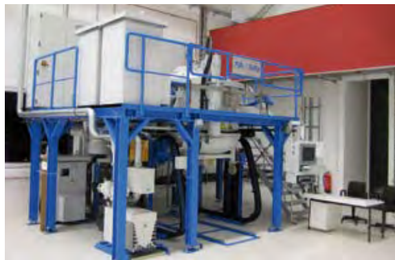
Fig. 1: Industrial crystallisation facility (VGF) to produce multicrystalline silicon ingots.
