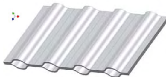
Fig. 3: Illustration of a heat-transfer structure for compression heat pumps using air as the heat source. The applied manufacturing process combines advantages from flat-pipe heat exchangers with lateral flow and conventional fin-pipe heat exchangers with longitudinal flow.
