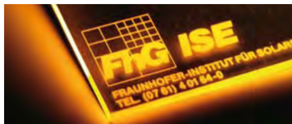
Fig. 5: This sample from the early years of Fraunhofer ISE demonstrates how the light is directed to the edges of the fluorescent concentrator.
